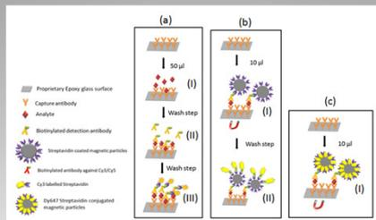
**Figure 1.** On-chip sandwich immunoassay steps for (a) the classical chip (b) the miniaturized chip and (c) the optimized miniaturized chip
