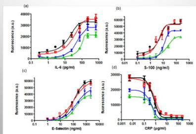
**Figure 2.** Calibration curves for (a) IL-6 (b) S-100 (c) E-Selectin and (d) CRP using the classical chip (→), the miniaturized chip (△), the classical chip + strept. MPs (●) and the miniaturized chip + strept. MPs (◆)
